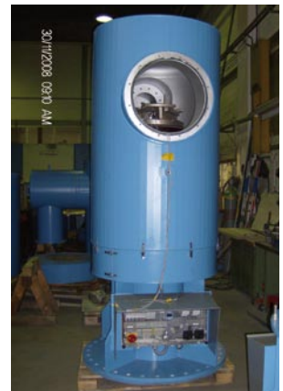
A dry insulation under fabrication
