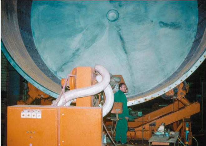
Homogeneous lead lining of an autoclave section
